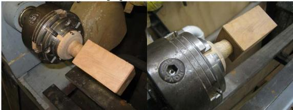
Bring up the tail-stock to support the blank and your are ready to start turning. Once the bulk of the material has been removed the tail-stock can be take away for final turning and sanding.
