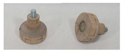
To prepare the blank drill an 8-8.5mm hole (M10 or 3/8" tapping hole size) in one end, approx 25mm deep, then thread using a standard M10 or 3/8" tap.
